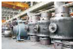
为西气东输三线（西段）制造的 31台48"，Class900高压大口径全焊接球阀 31pcs 48" 900# fully welded ball valves used on West-to-east Gas Transmission Pipeline Phase III
