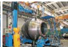
为天然气管道关键设备国产化研制的 56"，Class900高压大口径全焊接球阀 56" 900# fully welded ball valve made for home-made project of key equipments on natural gas pipeline
